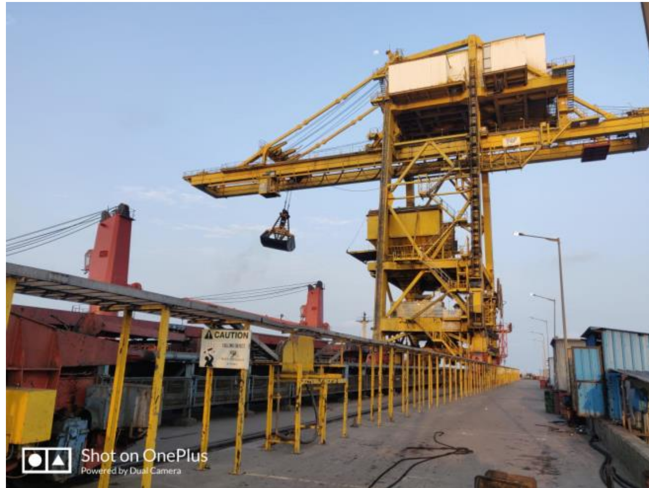
Grab Un-Loader (Capacity : 2 x 2000 MT/Hr) for Unloading of Coal from Ship
